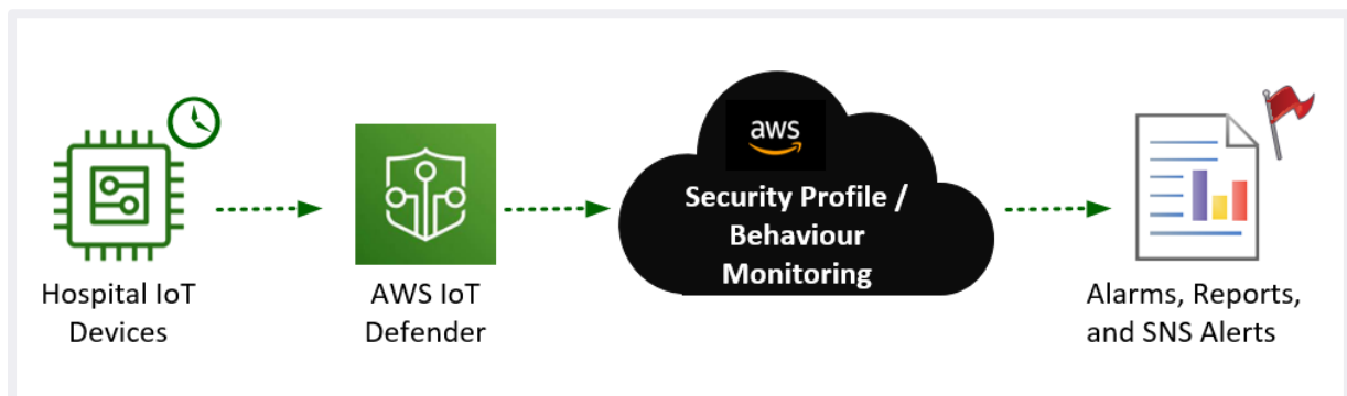
Figure 3. Defender utilises behaviour metrics and rules to create security profiles for monitoring IoT communications.
